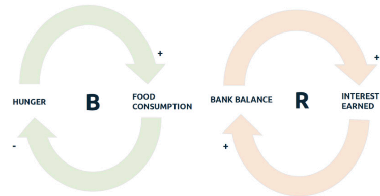
Figure 53: The most commonly used examples: the left loop is balancing, the right reinforcing
